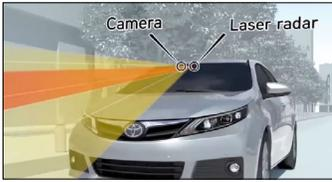
Toyota Safety Sense™ C<sup>2</sup> features three proprietary active safety technologies: Pre-Collision System<sup>3</sup>, Lane Departure Alert<sup>6</sup>, Automatic High Beams<sup>7</sup>. TSS-C<sup>2</sup> combines an in-vehicle camera and laser for outstanding performance and reliability. The package is designed to alert the driver to and/or help mitigate or prevent collisions in a range of vehicle speeds.
